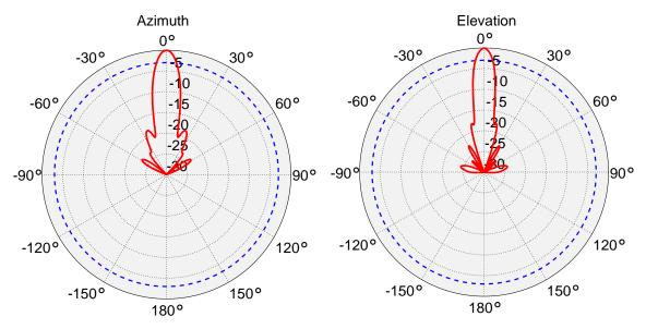
24 dBi Parabolic Antenna 3,500-3,800 MHz N Type Connector from L-com has same day shipment for domestic and International orders. Our portfolio includes coaxial cable assemblies, connectors, adapters and custom products as well as lightning and surge protectors, NEMA rated enclosures, and an RF product line which includes antennas, amplifiers, passive, and active components.
